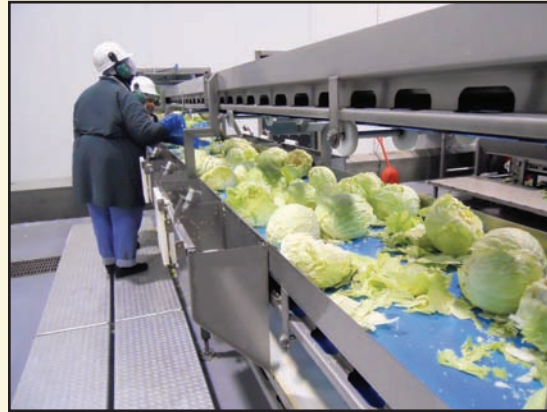
Prepackaged salad mix starts with giant vegetables like these massive heads of lettuce that have just had their cores removed. They move on to machines that cut, mix and fill the ingredients into controlled atmosphere packaging.
