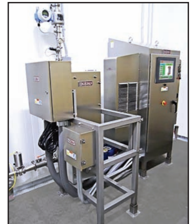
The BiIonix Costco installation. On the top left is a liquid flow meter, one of several sensors monitored by BiIonix's automated control system.
