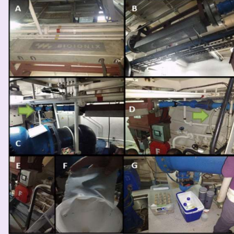
Fig.4. (A and B) Electrochemical reactor installed in wellboat. (C and D) The green arrow shows the hoses from where the samples were taken, before (control) and after (treatment) passing through the reactor. (E) Electrochemical reactor programming module. (F) 20 μm filter with retained A. catenella cells. (G) Flasks with samples of A. catenella .
